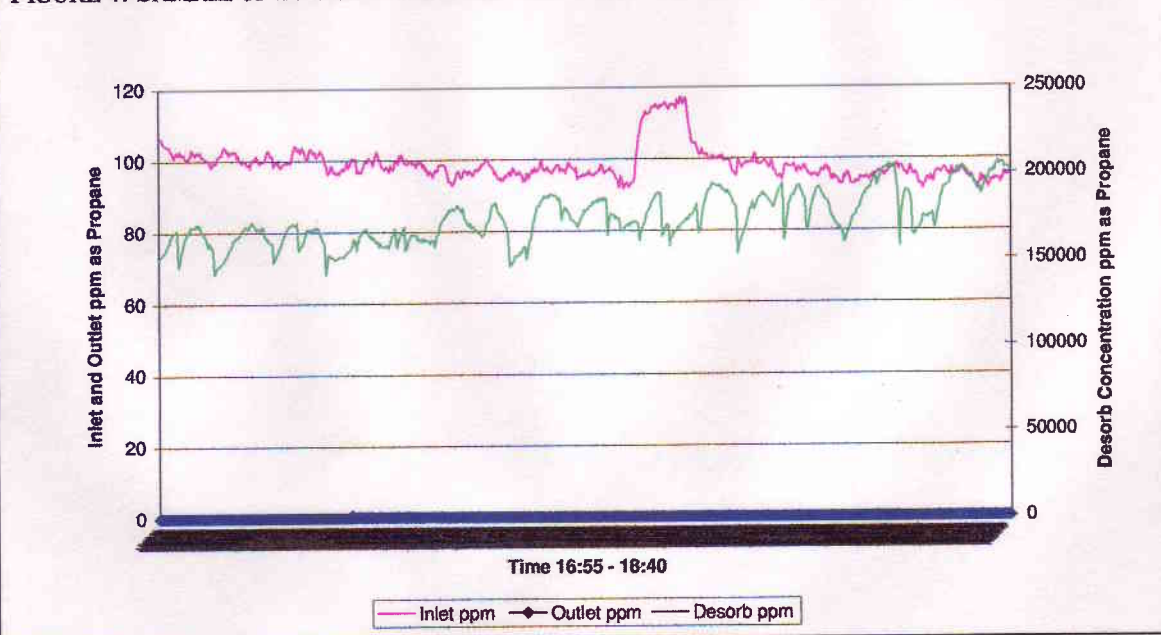
FIGURE 4: SAMPLE OF EMISSION TEST RESULTS FROM A FLUIDIZED BED CONCENTRATOR
